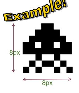
8px X 8px (64 pixels total) Only black and white used Single bit used to store each pixel 1=black 0=white
