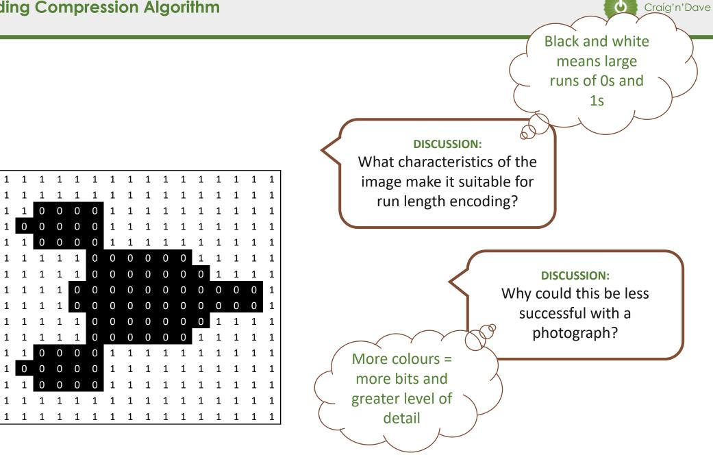
Consider this 16x16 pixel icon of a space ship that could be used in a typical computer game to represent a player life. A white pixel is represented with a 1. A black pixel is represented with a 0. The data is stored as a stream of 0's and 1's in a file. The file is currently 32 bytes.
